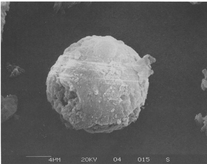
Fig. 2. Scanning electron micrograph of carbon CF19.
